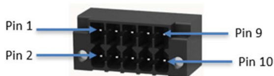
Figure 50: MCS connector (DEGSON 15EDGRHCM-THR-3.5-10P)
